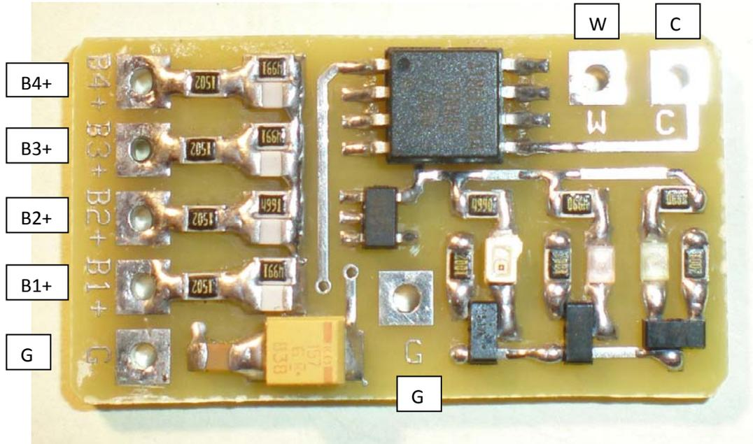
Connect the PCB V4.X as follows; voltages given are nominal for each cell, your may differ slightly.
